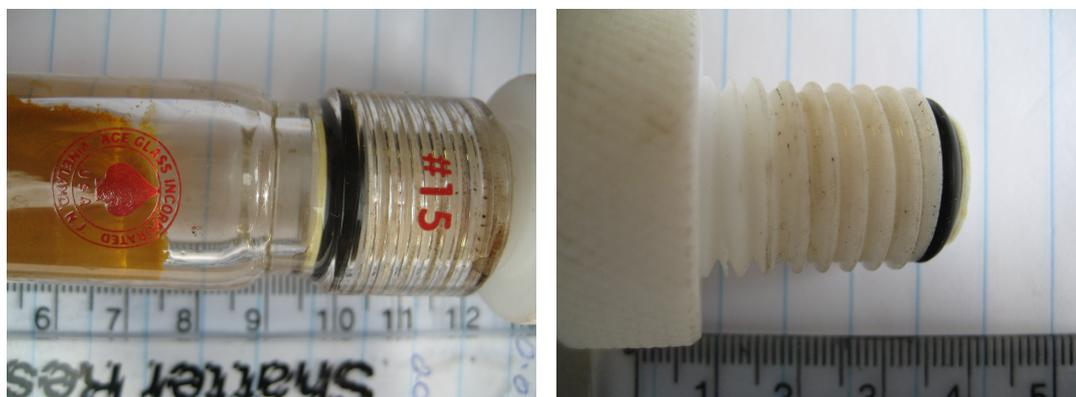
(a) An Ace Glass Pyrex tube (size #15) with (b) Ace Glass #15 PTFE screw top showing the a front mounted O-ring seal positioned at the thread. This was the only size used, though end of the PTFE screw top. Jarosite formation the thread itself was prone to deformation and that grew up the side of the Pyrex tube near replacement PTFE screw tops had to be made. to the PTFE screw top can be seen.
