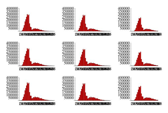
Spectra computed at the field locations. First row is top of scan (+25mm), lowest bottom of scan (-25mm). Left column is field center, rightmost is + 25mm field position.
