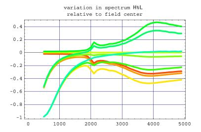
Difference between spectra at the field locations; the spectrum a the center of the field (leftmost in second row below) is taken as reference
